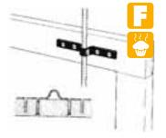
screws, 2 off 5 mm csk machine screws and tee nuts. As usual, during our testing we find the wood breaks well before the grummet is affected. Now available as self-colour for welding to steel frames.
