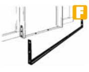
black. Size: Stated width between lugs plus 8 x 200 mm height. Fixings needed: No.10 [5 mm] csk screws or M5 csk machine screws.
